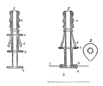
Cannula for measuring lateral pressure (longitudinal section).
